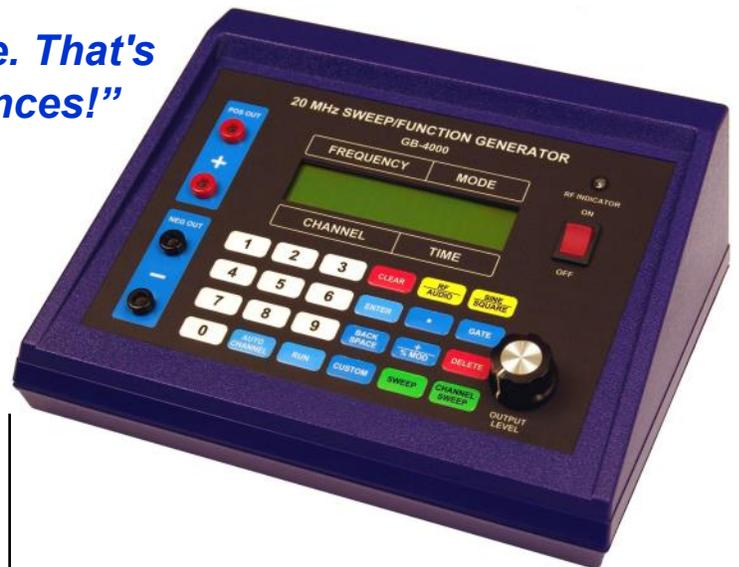
Step 1: Press the auto-channel button using the keypad.
